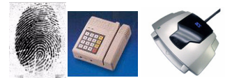
The locks are controlled by secure devices such as fingerprint scanners, proximity readers and smart card readers.
